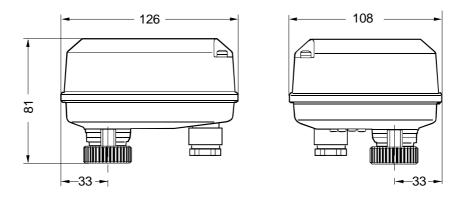
Fig. 1 Dimensions in mm
